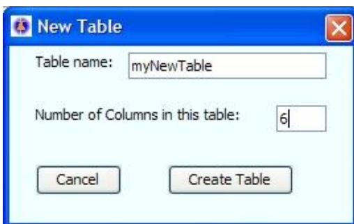
Figure 22: Creating a new database table. For example, table “myNewTable”, has six columns/fields once created.
