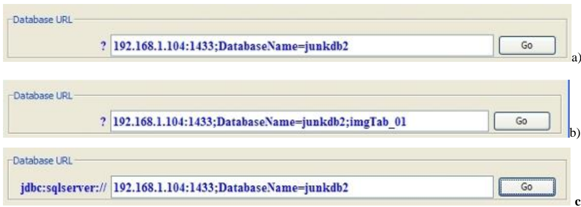
Figure 13: Typical connection procedure to Microsoft SQL. Database “junkdb2” specified (a), database and table “imgTab_01” specified (b), and final syntax (c). “DatabaseName” is not case sensitive.
