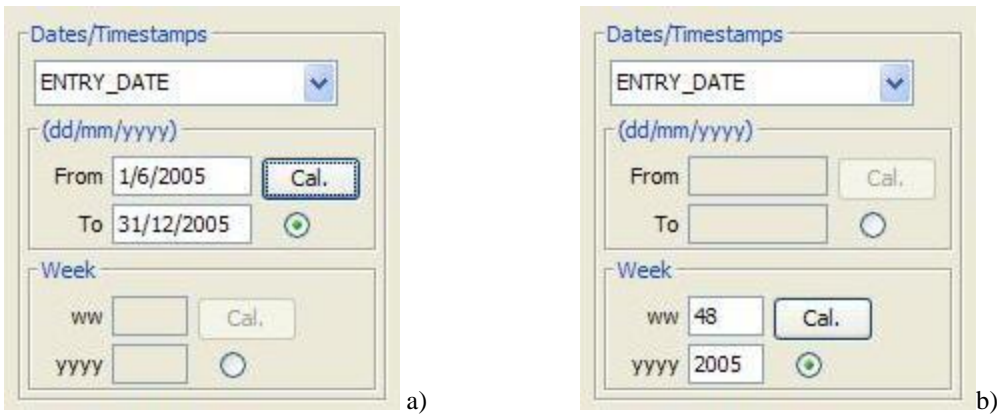
Figure 38: Queries with date (a) and week (b) clauses. Users can use the calendar “Cal” to specify the dates or the week. The first week in calendar starts on the first “Sunday” of the year.
