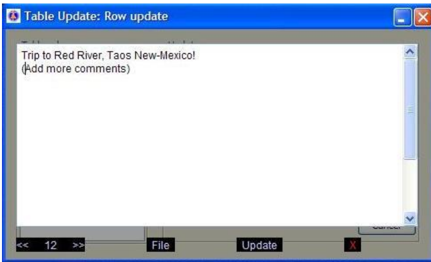
Figure 32: Text column update in database table. The utility includes a text editor. The text editor provides "font size", a button "File" for displaying the content of a file in user's hard drive, the "Update" button to initiate update process, and "X" button for closing the text editor.
